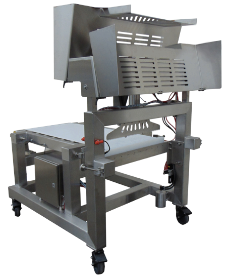
Flip open guards for complete access and easy cleaning
